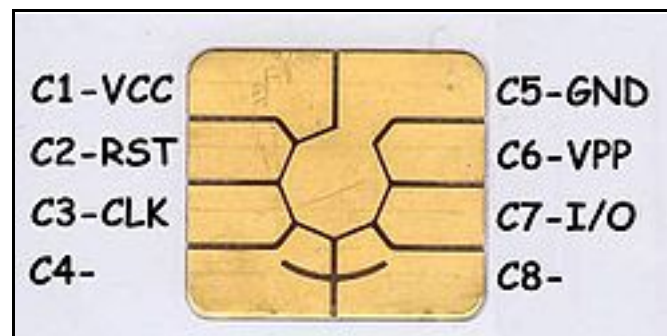
Gambar 2.6 Smart Card's pin contact (Anonim2)
